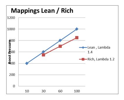
Having two mappings the requested boost pressure can be interpolated between the two curves in the graphic above.
