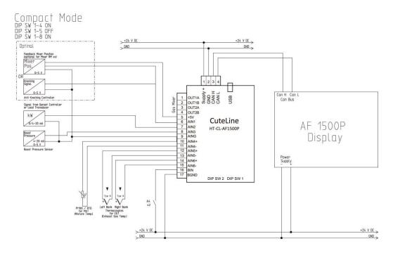
The AF 1500P Display shows all measured values and can be used for the setup.
