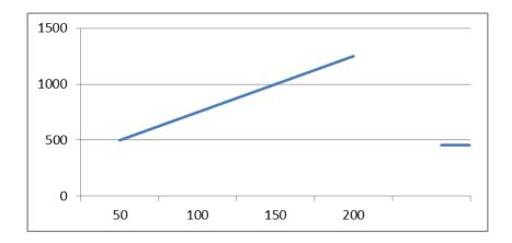
So the controller needs a mapping of load and boost pressure to be configured while commissioning. Once this mapping is set the mixer controls is controlled by the requested boost pressured (which is calculated by the actual load) and the actual boost pressure.
