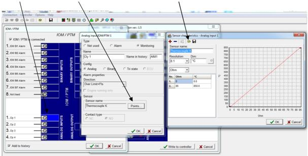
To be configured as Thermocouple K (°C) and Pt100 or Pt1000 (RTD) (°C), the ready sensor characteristics curve (CRV file) for these sensors can be downloaded from <a href="http://www.huegli-tech.com/">http://www.huegli-tech.com/</a>. For other type of sensors, the respective sensor characteristics curve must be created by the user accordingly.
