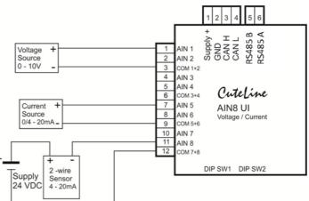
Note: Unused inputs must be connected to its corresponding COM x+y and the corresponding DIP switch must be OFF.
