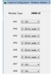
Launch the software and click on "Connect". Select the sensor type which is connected to the individual inputs and click on "Ok". If the configuration is successful, you will receive a pop up box message to notify you about it. After this is completed, click on "Disconnect" and turn off the power supply to the module. This completes the sensor type configuration process.
