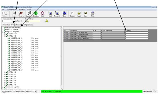
Digital Outputs → Select the appropriate DO\_DITEL\_# → Select the required function of this Output
