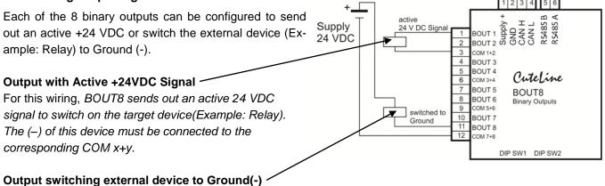
For this wiring, the target device (Example: Relay) has to be connected to a power supply(+) and the BOUT module corresponding input. The corresponding COM x+y must be connected to Ground.
