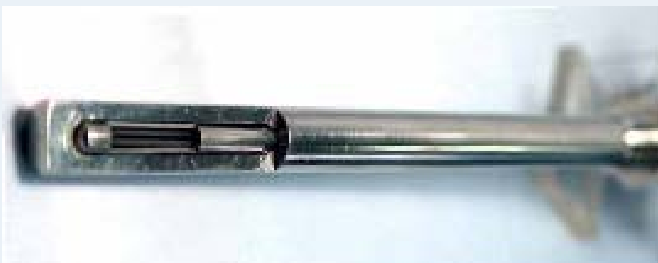
DESIGNED SENSOR WITH ELEMENT & PROBE COVERED WITH THERMOWELL
