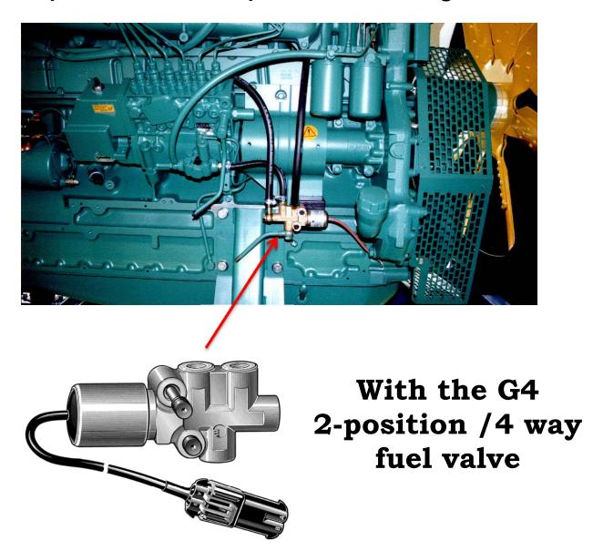
When an alarm signal occurs, the G4 fuel valve instantly reverses the supply pump suction into the injection pump.
