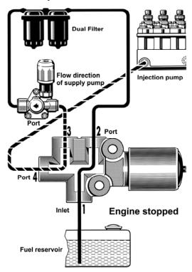
In this mode, the engine is stopped by energizing the Solenoid.
