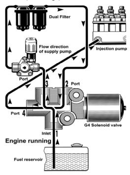
In this mode the supply pump aspirates the fuel from the reservoir into port "1" through to port "3", through the filters and via valve port "2" and outlet "4" into the fuel injection pump.
