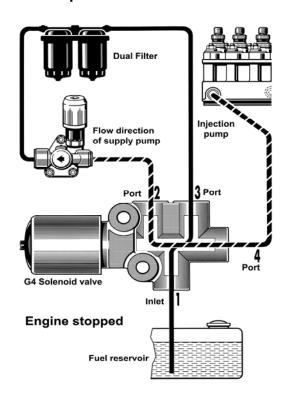
When the supply voltage is shut off, the valve spool instantly moves to Stop position.
