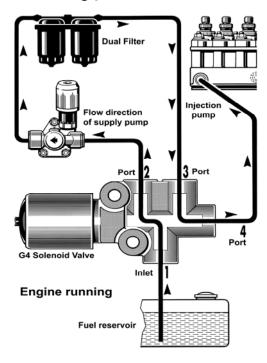
On the E.T.R. side of the valve the flow direction at the connecting ports is marked with arrows.
