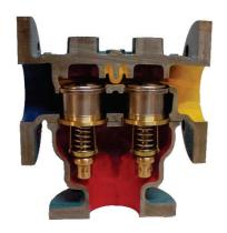
When the liquid reaches a predetermined temperature, the elements open and divert the flow to a different port.
