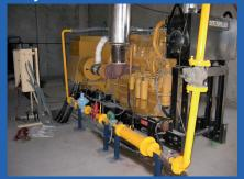
Custom specified conversion on a brand new CAT 3306 with CNG. Fuel ratio: 20% Diesel 80% Gas at 100% load. The engine was converted in our factory in Switzerland. Test conditions: Ambient temperature: 28°C, humidity:40% relative, resistive load bank.
