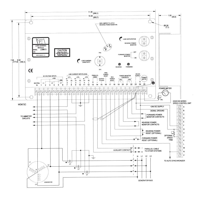
Terminals 1-6 accept for the 3 PHASE VOLTAGE inputs. Selection of the proper 3 terminals is dependent on the generator voltage. See Specification, page 2.
