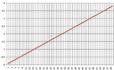
The graph shown above assumes a user can complete one cycle (1.22 cu. in. / 20 cm³) every 5 seconds (12 cycles per minute) and remain consistent during a period of 60 minutes. Please consult Huegli-Tech for theoretical recharging time for a specific application.
